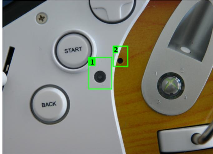
Figure 1.1: Calibration hardware present on some RB guitars, where (1) the light sensor and (2) microphone are highlighted [3]
